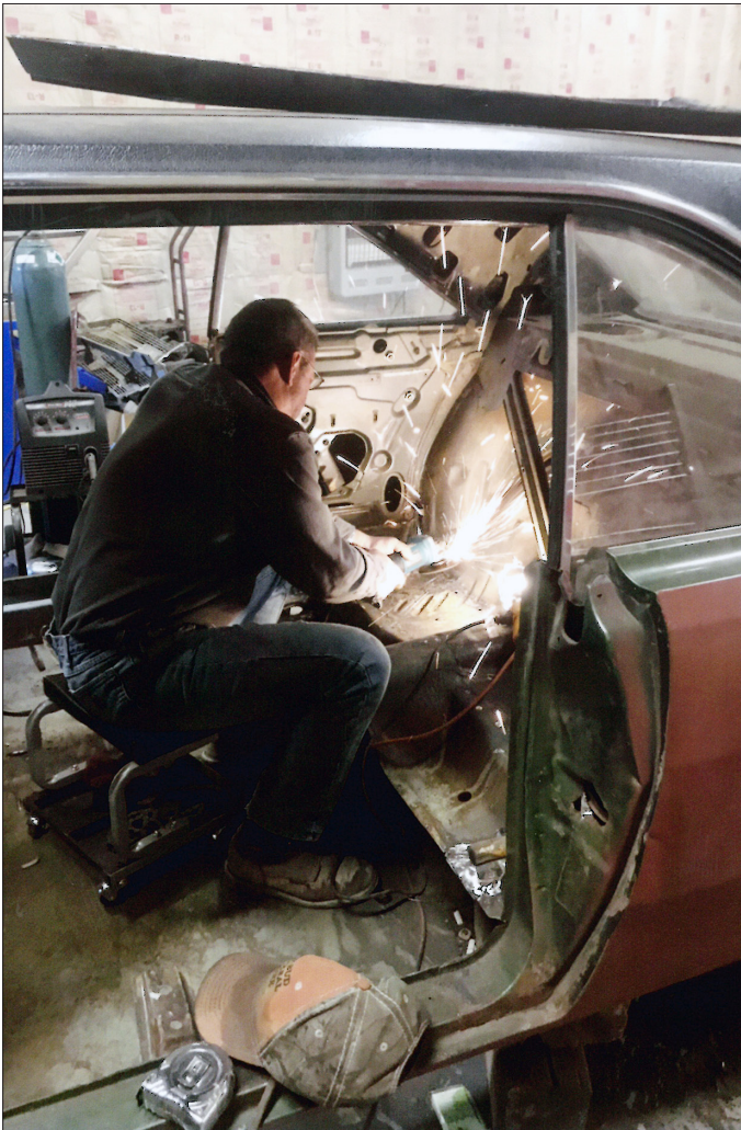
JAHNSEN USES a grinder on the back seat of the Dart Swinger(photo left). The bare metal (above) is ready for the primer. PHOTOS SUBMITTED
