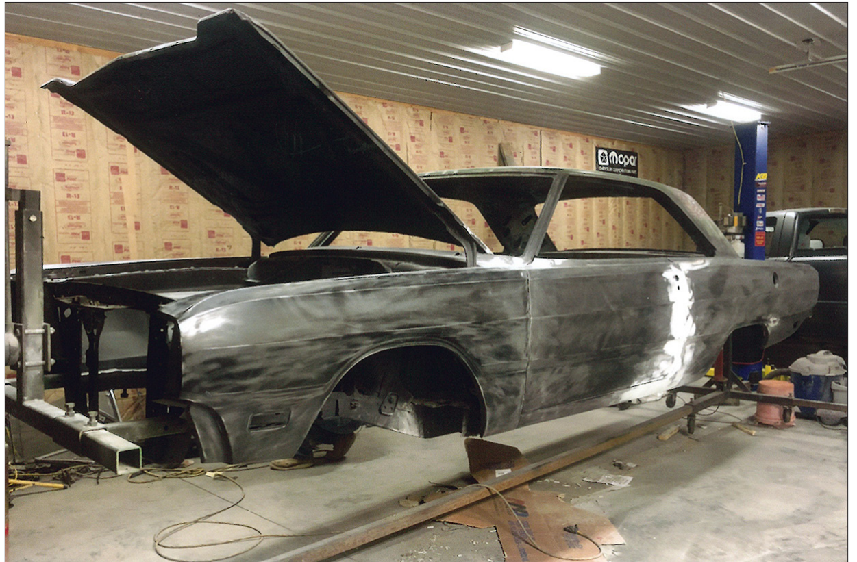
JAHNSEN USES a grinder on the back seat of the Dart Swinger(photo left). The bare metal (above) is ready for the primer. PHOTOS SUBMITTED
